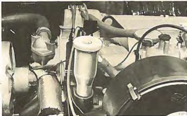
Oil filler cap, engine
