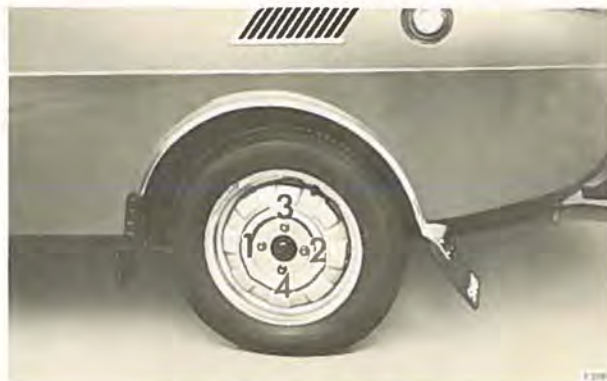
Order of tightening wheel nuts
