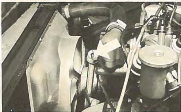
Location of dipstick, automatic transmission
